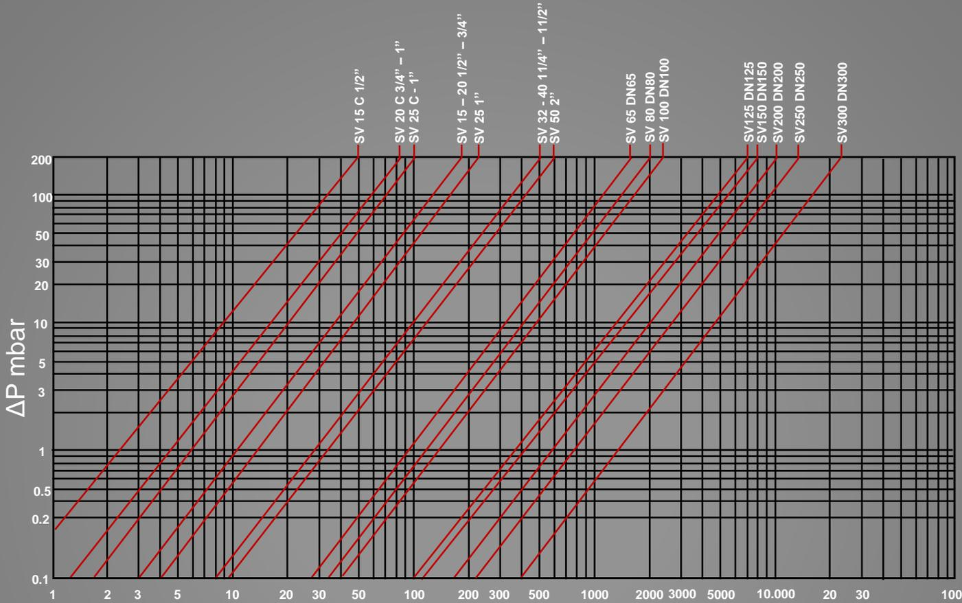
Debi Q (Stm3/h) / Flow Rate = Doğalgaz / Natural gas, Şartlar, Base: +15°C, 1013 mbar, kuru
